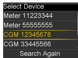
Select the **CGM device number that matches the serial number** located on the top of the inserter
