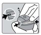
Free the tubing from the slot that holds it in place.
