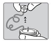
5. Make sure the top of the reservoir is dry. Gently push the tubing connector onto the top of the reservoir and turn it clockwise until it slides and locks into place.
