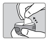
Squeeze the three raised markings on both sides of the mio lid. Lift and remove the lid.
