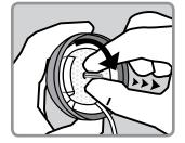
Place the tubing in the slot on the side of the inserter.
