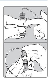
Turn the plunger counterclockwise to unscrew it from the reservoir.
