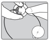
4. Make sure the top of the reservoir is dry. Gently push the tubing connector onto the top of the reservoir and turn it clockwise until it slides and locks into place.
