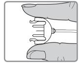
3. Slide the set release connector into the set connector.
