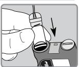
2. Turn the tubing connector clockwise until it locks into place.
