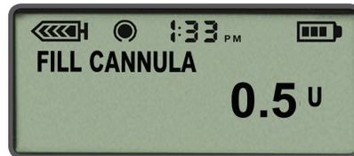
**Note:** Fill Cannula is to fill the empty cannula after the insertion needle has been removed. The tubing is already filled.
