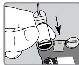
2. Turn the tubing connector clockwise until it locks into place.
