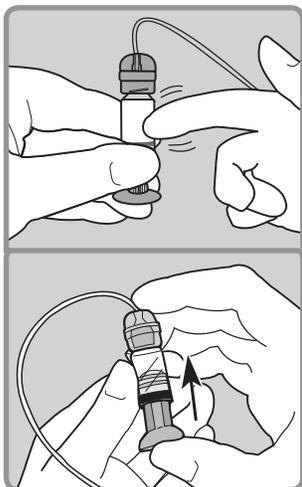
4. Turn the plunger counter-clockwise to unscrew it from the reservoir. Be careful not to pull the plunger before it is disconnected, or insulin will spill out.
