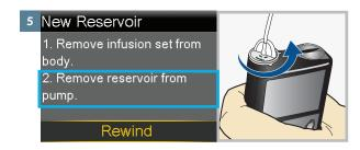
Remove the used reservoir from the pump.
