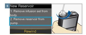
Remove the used reservoir from the pump.
