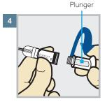
Twist plunger counter-clockwise to loosen and remove.
