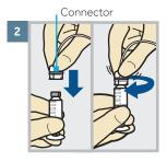
Gently push the tubing connector onto reservoir. Turn clockwise until locked. You will hear a click.
