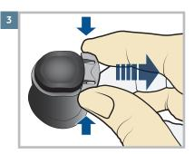
Remove the disconnect cover (the small plug below the button) by gently squeezing the sides of the disconnect cover then pulling it away from the insertion device.
