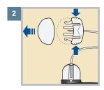
Remove the white cap from the site connector by squeezing the sides of the site connector then pulling the white cap off.
