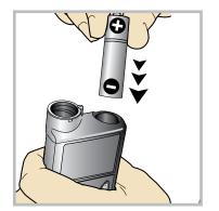
**STEP 1.** Place the battery into the battery compartment with the negative (flat) end going in first.
