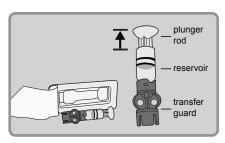
2. Pull plunger rod down to fill reservoir with air.
