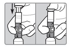
5. Continue to hold plunger rod down as you turn vial over (vial should now be on top and reservoir on bottom). Release plunger. Then slowly pull plunger rod down to fill reservoir with insulin.
