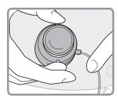
4. Press the two white buttons at the same time. If they are not pressed at the same time the Quickset® will not insert properly.
