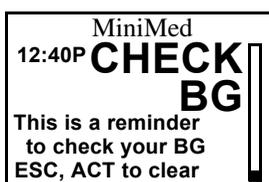
When the BG reminder goes off, your pump will beep or vibrate and the message “CHECK BG” will appear on the screen. Your pump will beep or vibrate periodically until it is cleared (**ESC, ACT**).
