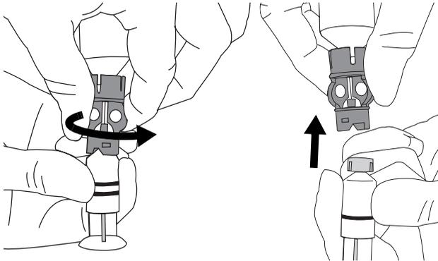
**9.** Put the tubing connector on the reservoir. Turn it clockwise to secure.
