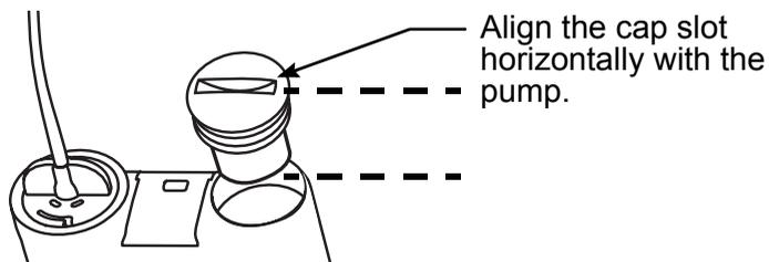
5. Turn the battery cap clockwise 4 half-turns so the slot is aligned horizontally with the pump as shown here:
