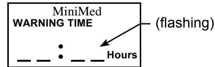
The pump will alarm first when the specified time remains, then again one hour before empty.
