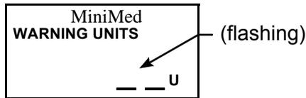
The pump will alarm first when the specified units remain, then again when half that remaining amount is used.
