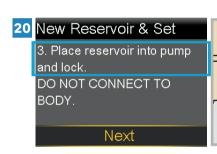
Place the reservoir into the pump. **Do not** connect the infusion set to the body.
