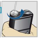
Remove the used reservoir from the pump.
