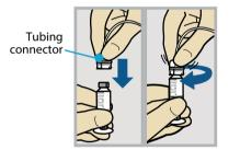
Gently push the tubing connector onto the reservoir. Turn the connector clockwise until it is locked into place.
