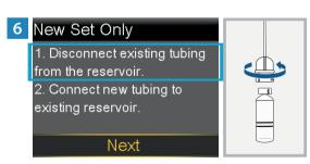
Disconnect the tubing connector of the used infusion set tubing from the reservoir. Place the reservoir on a clean surface. Do not throw the reservoir away.
