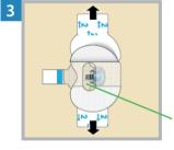
Remove the liner marked 2 from each side.
