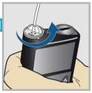
Remove the used reservoir from the pump.
