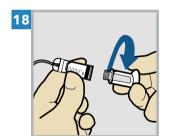
Twist the plunger counter-clockwise to loosen it and to remove it.
