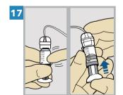
Tap the reservoir to move any air bubbles to the top. Push the plunger slightly to move the bubbles into the tubing.
