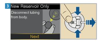
Disconnect the tubing from the cannula housing. Do not remove the cannula housing from the body. Select **Next**.
