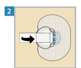
Cover the transmitter with the adhesive tab.
