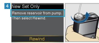
Remove the reservoir from the pump.
