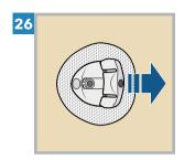
Remove the disconnect cover by squeezing the sides and pulling away from the cannula housing.
