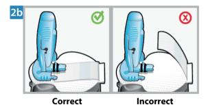
**Tuck the adhesive tab**. Make sure that the sensor's adhesive tab is tucked under the sensor connector and snaps.
