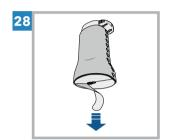
Remove the paper backing from the adhesive. Be careful not to touch the adhesive.
