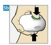
**Insert the sensor**. Press the **bump** on both buttons and release them at the same time.
