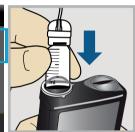
Place the reservoir into the pump. **Do not** connect the infusion set to the body.
