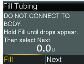
2. Select and hold **Fill**. Your pump beeps six times as it dispenses insulin into the tubing toward the infusion set needle. Continue to hold **Fill** until insulin droplets form on the tip of the infusion set needle, and then release. Your pump beeps as it fills the tubing, and the amount of insulin used appears on the screen.
