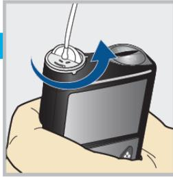
Remove the used reservoir from the pump.
