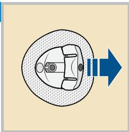
Remove the disconnect cover by squeezing the sides and pulling away from the cannula housing.
