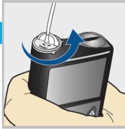
Remove the used reservoir from the pump.
