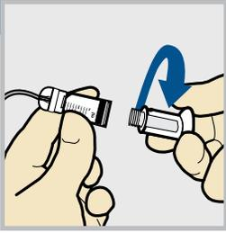
Twist the plunger counter-clockwise to loosen it and to remove it.
