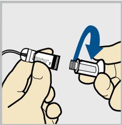
Twist the plunger counter-clockwise to loosen it and to remove it.
