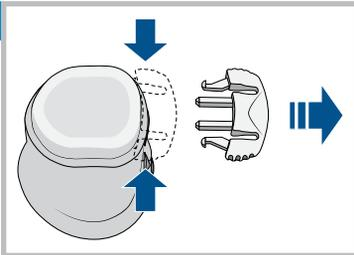
Remove the disconnect cover from the insertion device by gently squeezing the sides of the disconnect cover then pulling it away from the insertion device. Keep the disconnect cover for later use.
