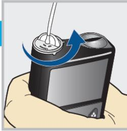
Remove the reservoir from the pump.
