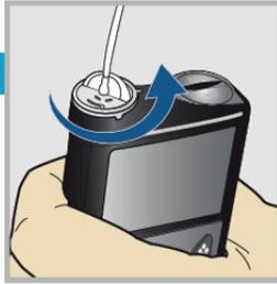
Remove the used reservoir from the pump.
