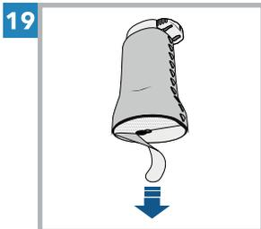
Remove the paper backing from the adhesive. Be careful not to touch the adhesive.
