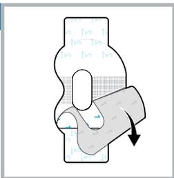
To apply the 2nd tape, remove the liner marked 1.
