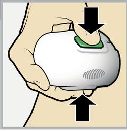
**Insert the sensor.** Press the **bump** on both buttons and release them at the same time.
