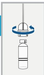
Disconnect the tubing connector of the used infusion set tubing from the reservoir. Place the reservoir on a clean surface. Do not throw the reservoir away.
