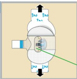
Connector and snaps in hole of tape.
