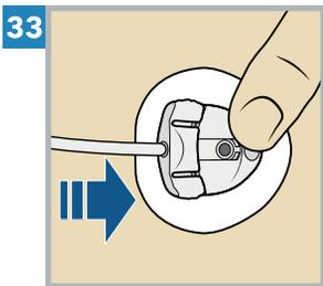
33 Gently hold the cannula housing steady with your finger. Then push the site connector straight into the cannula housing until you hear a click.
