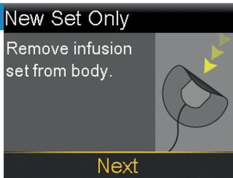
Remove the entire infusion set by loosening the adhesive and pulling the set away from the body. Select **Next**.
