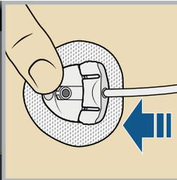
Use your finger to gently hold the cannula housing steady. Push the site connector into the cannula housing until you hear a click.
