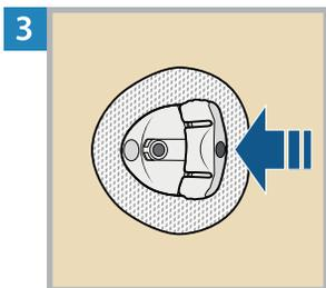
Put the disconnect cover on the cannula housing. Then push the cover into the cannula housing until you hear a click.
