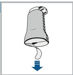
Remove the paper backing from the adhesive. Be careful not to touch the adhesive.
