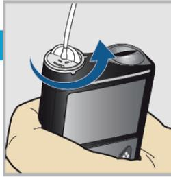
Remove the used reservoir from the pump.
