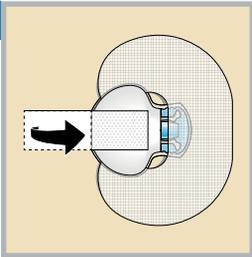
Cover the transmitter with the adhesive tab.
