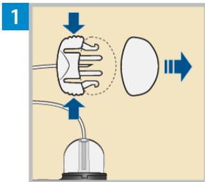
Remove the white cap from the site connector by squeezing the sides of the site connector then pulling the white cap off. Check to make sure there is no air in the tubing. If there is air in the tubing, fill the tubing with insulin as instructed earlier in this document.
