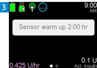
**Sensor warm up X:XX hr** will appear on the Home screen. After the warm up is complete, the pump begins receiving SG readings.
