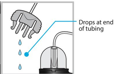
Select **Fill** and keep holding
