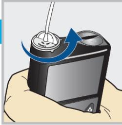
Remove the reservoir from the pump.
