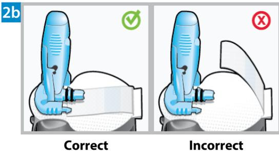
**Tuck the adhesive tab.** Make sure that the sensor's adhesive tab is tucked under the sensor connector and snaps.
