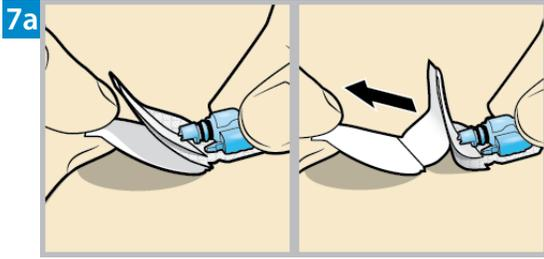
**Remove the adhesive pad liner.** Hold the sensor in place and gently remove the liner from under the adhesive pad.
