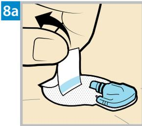
**Untuck the adhesive tab.** Untuck the adhesive tab from under the sensor connector.
