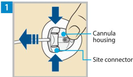
To disconnect, gently hold the cannula housing steady with a finger. Then squeeze the sides of the site connector and pull it out from the cannula housing.
