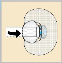
Cover the transmitter with the adhesive tab.
