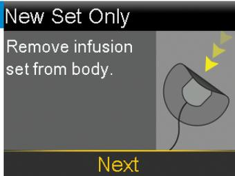
Remove the entire infusion set by loosening the adhesive and pulling the set away from the body. Select **Next**.
