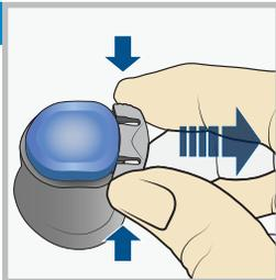
Remove the disconnect cover by gently squeezing the sides and pulling it away from the insertion device.
