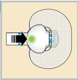
Connect the transmitter to the sensor.
