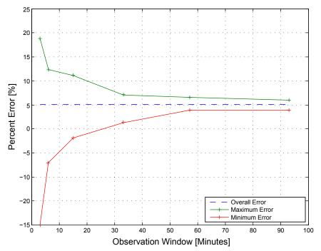
Trumpet Curve for MMT-1780 at intermediate rate of 1 U/h
