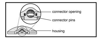
Look inside the connector opening of the transmitter to make sure that the connector pins are not damaged or corroded. If the connector pins are damaged or corroded, the transmitter cannot communicate with the charger or pump. Contact the 24 Hour HelpLine. It may be time to replace your transmitter.
