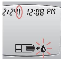
The meter will turn on. A test strip with a flashing blood drop will appear, letting you know the meter is ready to test, and the Send arrow (↑) will show that the meter is set to send the result to your compatible Medtronic device.
