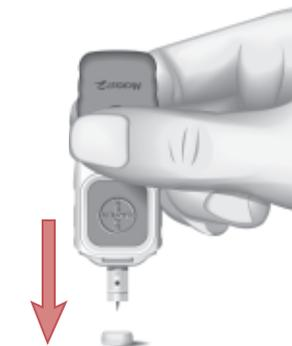
While (a) pressing the blue release button, (b) pull the blue cocking handle, and the lancet will drop into the container you have selected.
