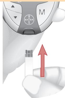
Hold the test strip with the gray end facing up.
