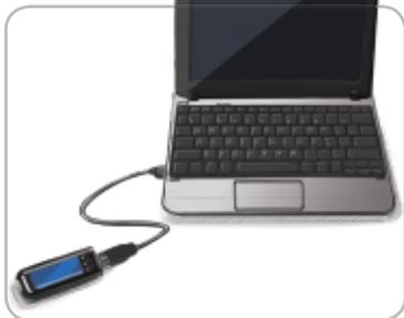
**You cannot do a blood glucose test while the battery is charging.** When charging is finished, the test strip port light will turn off. Unplug your CONTOUR NEXT LINK meter to test.
