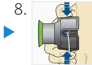
8. Press the two **green** side buttons at the same time. If they are not pressed at the same time the infusion set will not insert properly.
