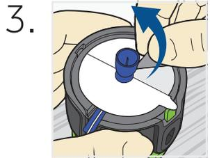
3. Peel the paper from the adhesive on both sides of the needle guard.
