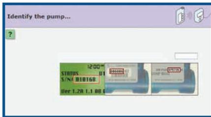
**5** Enter your pump's serial number as instructed on the **Identify the pump** screen.
