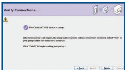
**7** **CONNECT** your USB linking device to your computer. The **Verify Connections** screen will appear to confirm communication between your devices and inform you when setup is complete. Click **Finish** to continue. **NOTE:** MiniMed 630G users, you will be prompted by the pump to **Connect Device**. Select **Yes** on your pump to allow connection.
