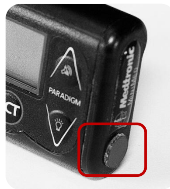
Loose Drive Support Cap- Cap sticking out
