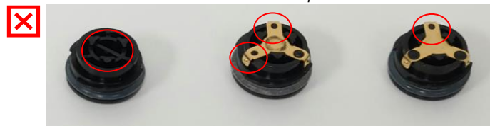
Damaged battery caps - Do not use
