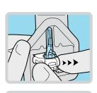
2. To load serter, push serter all the way down onto sensor and pedestal until serter sits on table.
