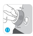
Grab center of inserter only, and gently pull to remove inserter from injection port.
