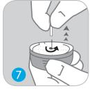
Twist and remove needle guard from introducer needle.
