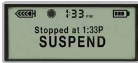
Pump in SUSPEND; notice the alarm icon
