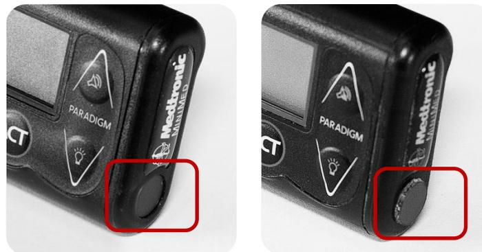
Normal Drive Support Cap- Cap slightly indented      Loose Drive Support Cap- Cap sticking out
